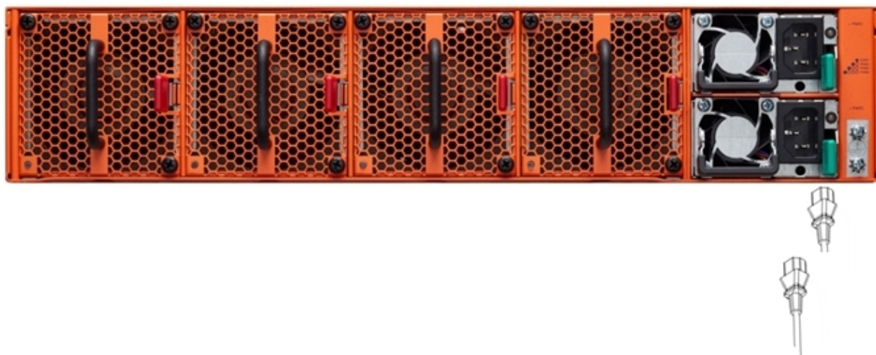
Figure 9 Connecting AC Power on a GigaVUE-TA25
